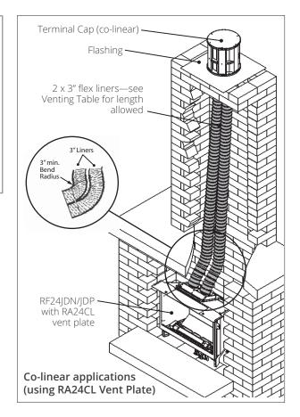
approved components (see *Approved Venting Components* in fireplace's Installation Manual) and proper vent clearances to combustibles must be maintained.
