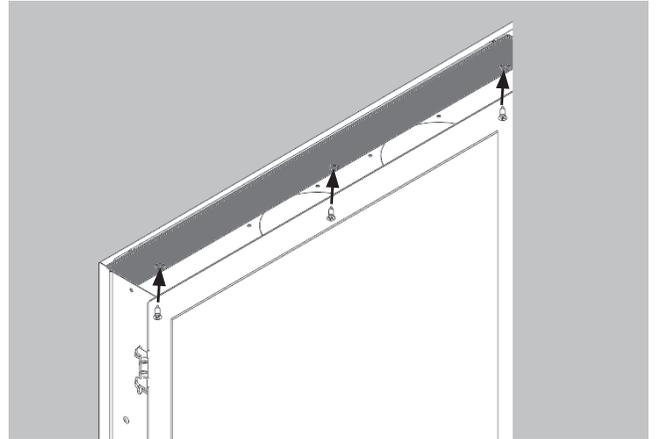
2. Locate the backing plate assembly inside the perimeter of the appliance's opening and press it firmly against the wall, as far as it will travel. Secure the plate using 4 black low profile screws (included).
