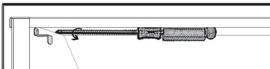
4. Place the rear panel against the back of the firebox, on the ledge at bottom.
