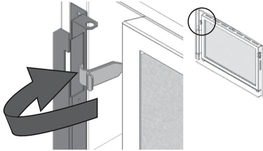
2. Place the window in its bottom railing and push its top against the firebox. **Ensure to remove any coal particles in the railing before installing the window.**
