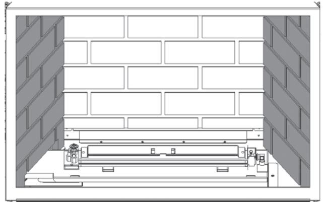
7. Tighten the side brick anchors on each side of the firebox.
