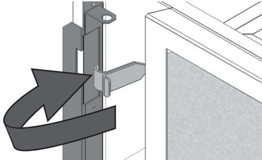
2. Place the window in its bottom railing and rotate its top against the firebox. **Ensure to remove any coal particles in the railing before installing the window.**
