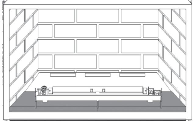
10. Reinstall the rear log support (3 screws). Its rear edge rests on the rear brick support ledge.
