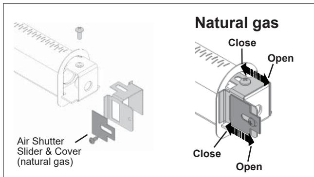
In a few unusual installations, the flame picture may be improved by adjusting the aeration. The need for adjustment should be determined only by operating the appliance with the ceramic logs and window installed.
