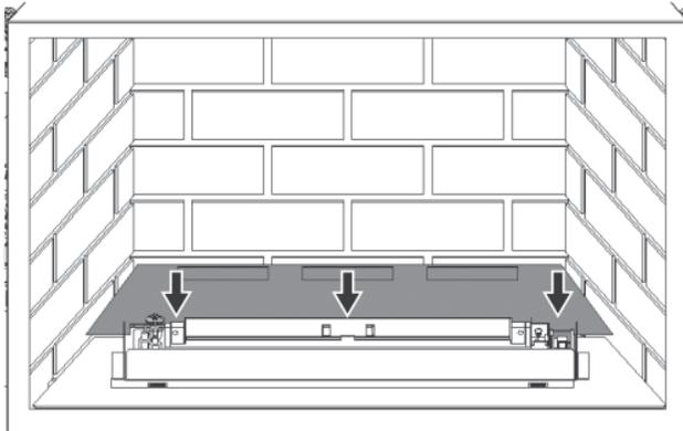
12. **With logs only:** Slide the cast iron grate in the slots in front of the burner.
