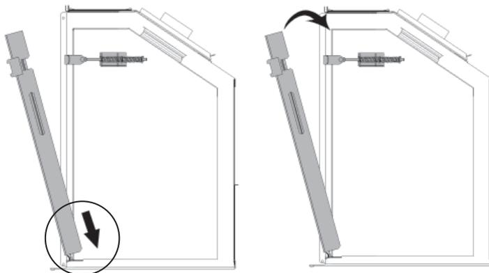
3. While you hold it, unhook the side levers from the side shrouds and hook them into the window brackets on each side.
