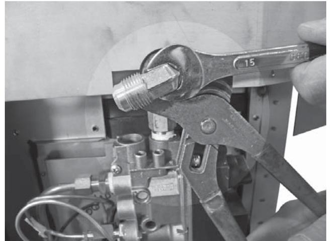
4. Install the flex connector to the alternate elbow.
