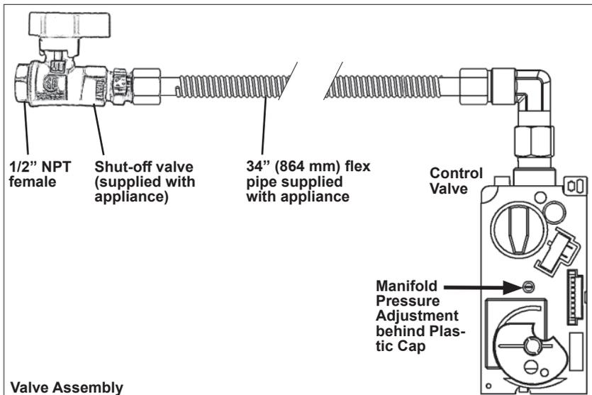
The appliance must be isolated from the gas supply piping system by closing its equipment shut-off valve during any pressure testing of the gas supply piping system at test pressures equal to or less than 1/2 psi (3.5 kPa).
