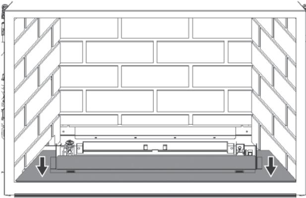
11. **With logs only:** Install the front bricks in front of the burner.
