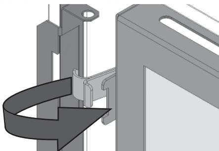
4. Pull out the top of the window and release it to ensure the springs return it.
