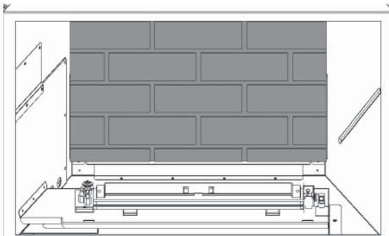
5. Rotate the anchor up and out of the way and slide the left hand side panel against the firebox side. Rotate the anchor back down to hold the panel.
