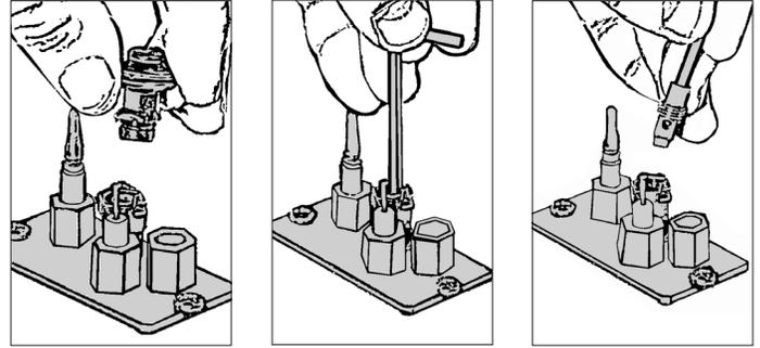
4. Refit the pilot hood by pushing down on it (it is keyed to only fit in one orientation). Ensure that it snaps into position.
