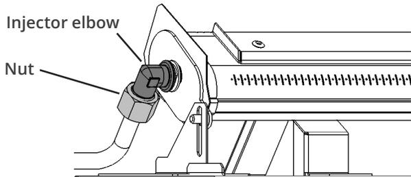
3. Unscrew and disengage the injector elbow. Be aware that **four pieces sit between the elbow and the burner, do not drop them.**
