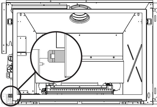
2. Adjust the aeration lever as required. Depending on fuel bed used, altitude and other considerations, the flame picture may be improved by adjusting the aeration. The need for adjustment should be determined only by operating the appliance with the fuel bed, liners and window installed and evaluating the flame picture after a 15-minute warm-up.
