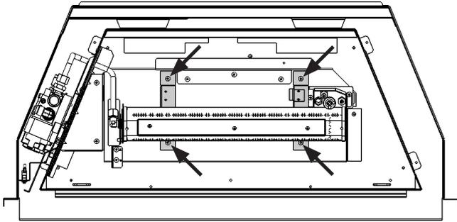
2. Unscrew the nut at the end of the burner fuel supply line, and lift the burner and supports out of the fireplace (complete with injector elbow attached).
