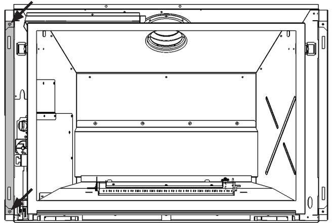
6. Remove the side cover (2 screws at left, 3 at the front).
