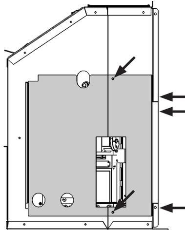
7. Remove burner cover (2 screws).
