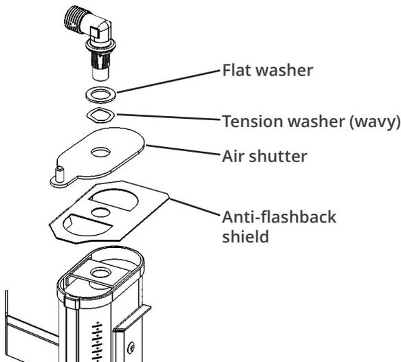
6. Replace the burner. The stem on the end of the air shutter must mate with the vertical slot in the link bracket. No nut is required.
