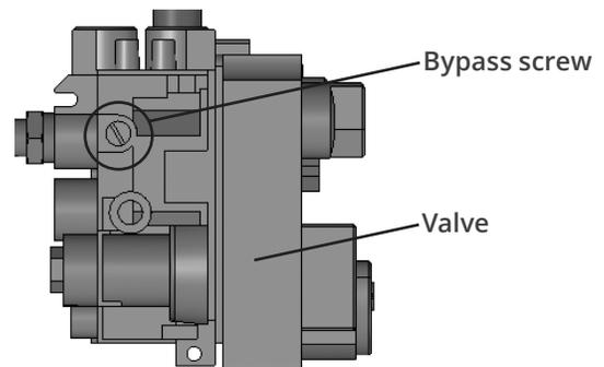
2. Insert the replacement minimum rate bypass screw and hand tighten using a screwdriver/Allen key. Refer to the *Specifications* table on page 1 for proper bypass screw (the number is stamped on the barrel of the screw).
