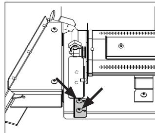
2. Rotate the stopper into the correct position for your desired gas. The initial of the desired gas will be toward the rear of the fireplace ("N" for Natural Gas, "P" for Propane). Pictured below: Natural Gas position on the left, Propane position on the right.
