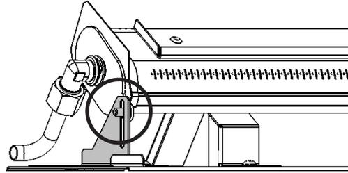
7. Connect the fuel supply line and tighten the nut. The burner may be adjusted to align the injector with the fuel line.
