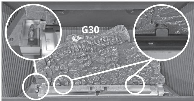
2. Place the base panel log on top of the burner, ensuring the vertical flange of the burner is inserted in the groove under the log as indicated.
