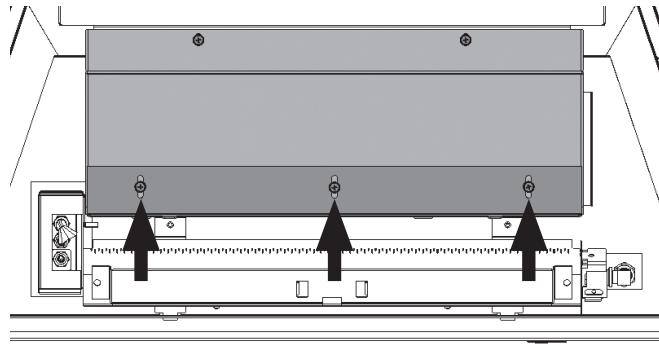
2. Install the fuel bed support bracket supplied with the log set, securing it re-using the same screws. Ensure the screws are centered in the bracket's slots as shown.
