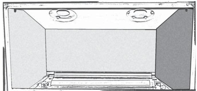
7. Tighten the side panels anchors on each side of the firebox.
