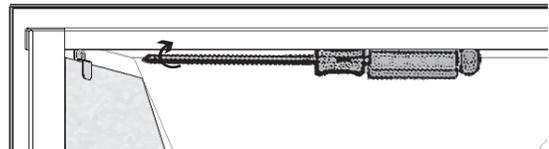
8. Install the port cover fixing it using the two screws already in the firebox top.
