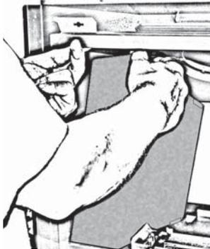
Rotate anchor up and insert panels
