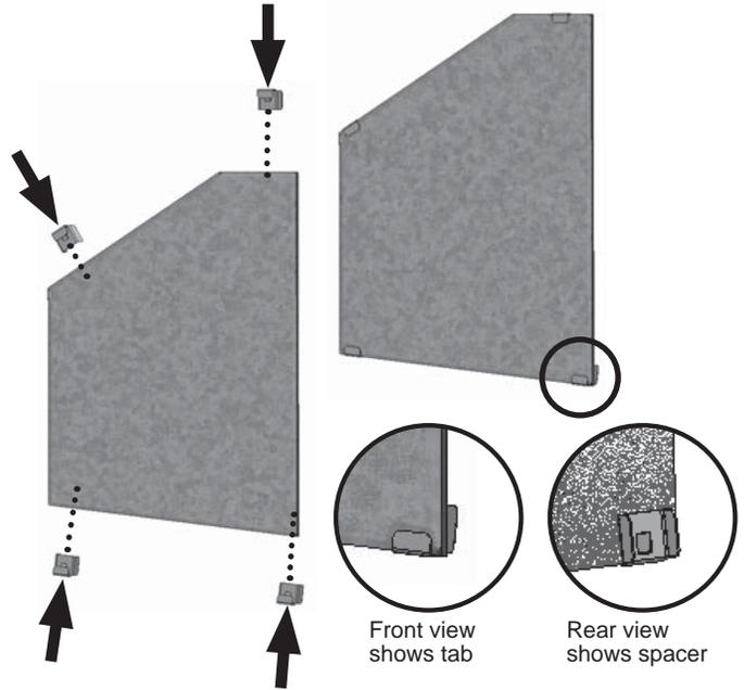
6. Rotate the anchor up and out of the way and slide the right hand side panel against the firebox side. **The panel should be parallel to the edge of the burner plate.** Rotate the anchor back down to hold the panel.
