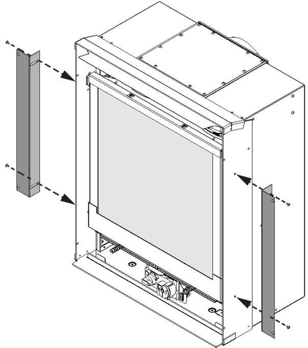
4. **Required for installation in combustible construction.** Bend the stand-offs into shape and fix them to the appliance's case as indicated (4 screws/side, pre-fitted on engine).
