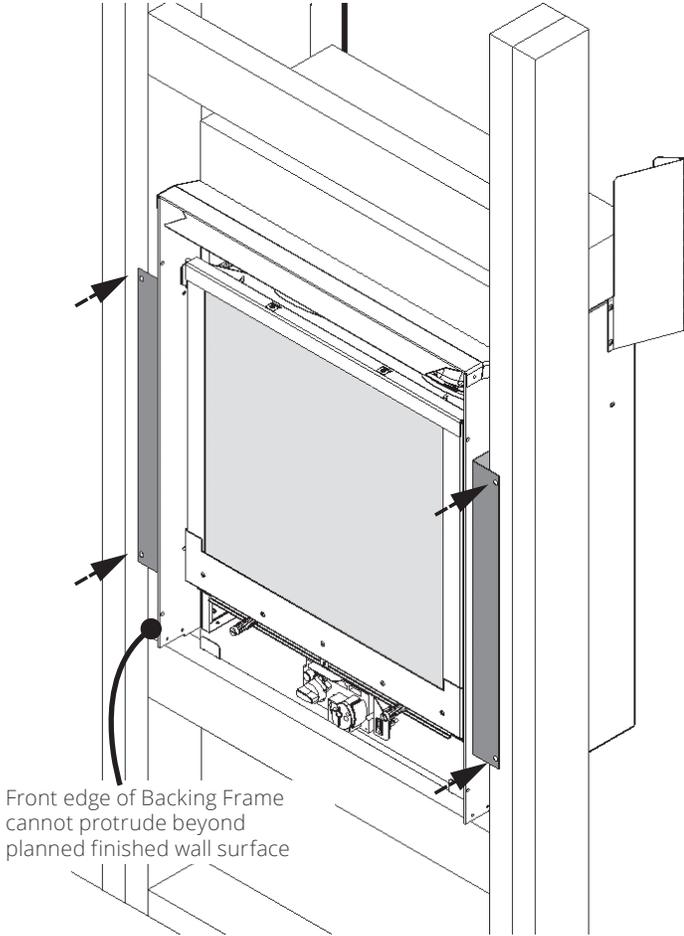
7. Fix the non-combustible cement board to the header and side studs of the frame. The board does not touch the top of the appliance—leave approximately 1" gap.
