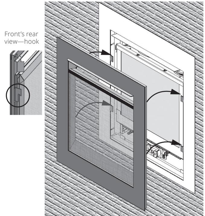
15. Slide the heat exchanger cover onto the heat exchanger. Note its shape and orientation.
