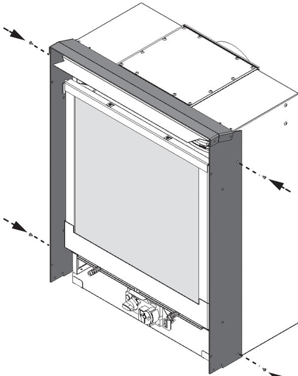
3. Install stud brackets over top of the backing plate frame assembly with 2 screws per side. See *Adjustability of the Ledgeview Front ZC section* for more information on position of brackets.
