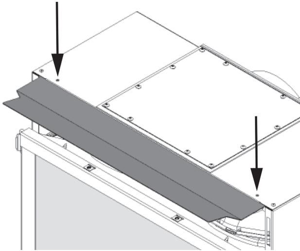
2. Slide the backing plate frame assembly over the appliance case and secure it with 4 screws provided.
