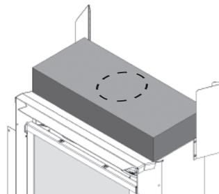
6. Insert the appliance into the framing and secure the stud brackets with two wood screws per side (not supplied). **Make sure the framing is leveled.**
