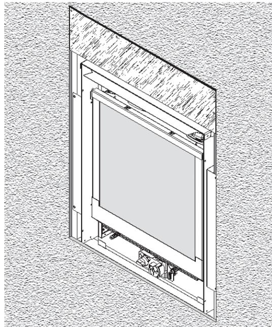
14. Insert backing plate within the frame assembly. Push plate over wall finish and secure it with two screws per side using the hole or slot at the sides depending of the wall thickness.
