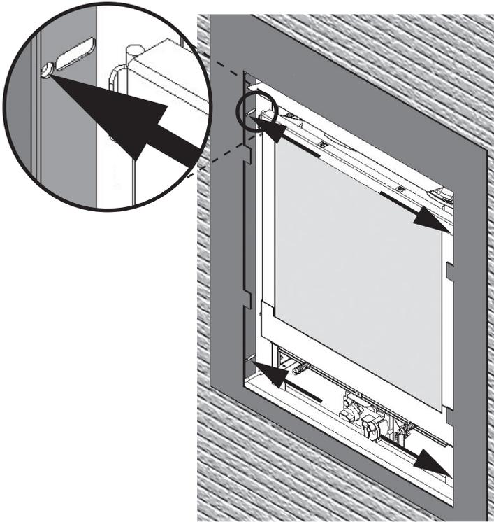
16. Hook the Ledgeview front assembly to the backing plate flanges.
