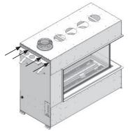
6. Place fireplace against the wall (with standoffs and support bracket between studs). Remove carrying handles before moving the fireplace into final position.
