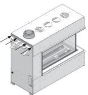
6. Place fireplace against the wall (with standoffs and support bracket between studs). Remove carrying handles before moving the fireplace into final position.
