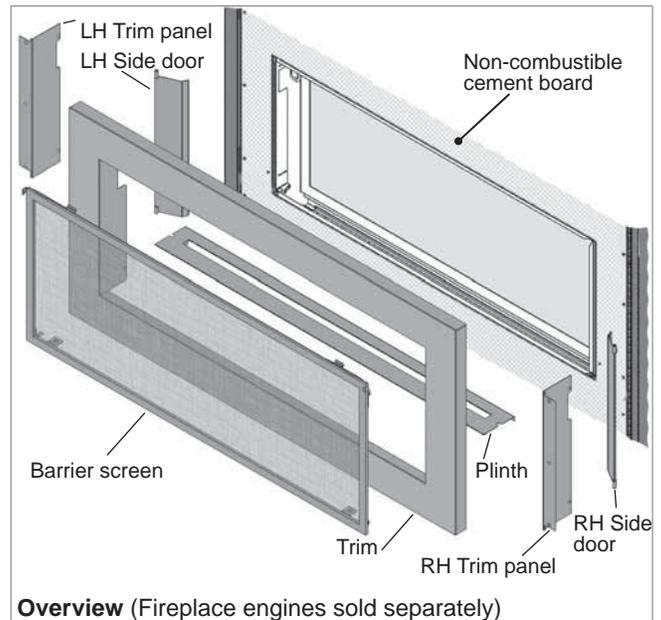
The 1750 Linear 5-1/4” Surround Kit is designed to be used on the Linear L2 1700 Valor heater.
