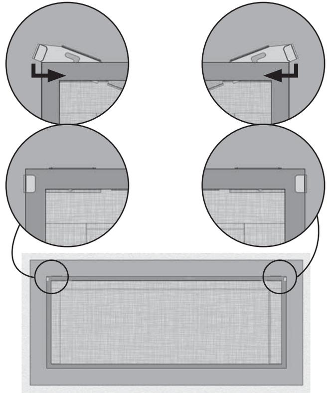
5. Verify that the screen is properly hooked to the trim and secure.
