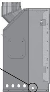
3. In the front left corner of the appliance case, slide the junction box tab into the slot of the appliance case located right behind the cable clamp. Ensure the wires are not pinched between the junction box and the appliance case..
