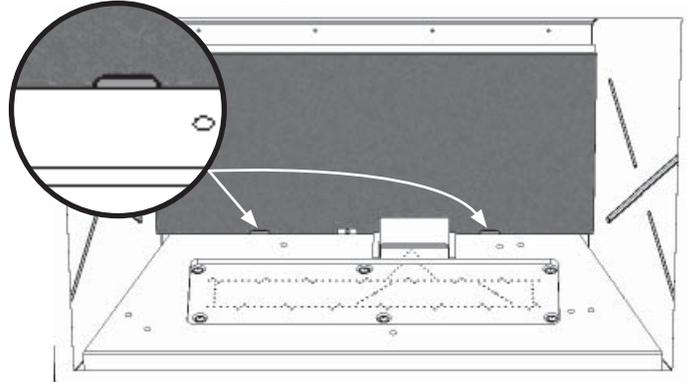
4. Install either the left or the right side glass and filler panels assembly against the firebox side and slide it back against the rear panels.
