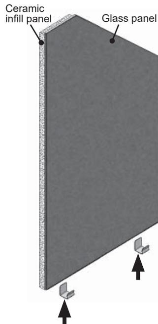
5. Rotate the side anchor over the top edge to hold the panels ensuring the panels are tight together. Tighten the anchor screw.
