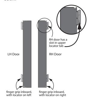
6. Position LH door to left side of front panel, identify door slots top and bottom just behind front panel and slide door locator in position.
