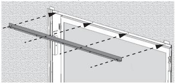
2. Carefully position and secure steel front panel with 4 low profile screws to 4 firebox mounting brackets. Before tightening, hold panel up against wall finish then tighten.
