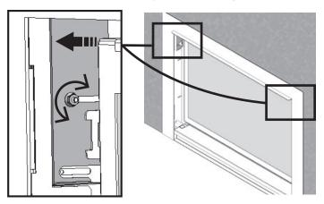
5. Identify left hand door from right using diagram below.
