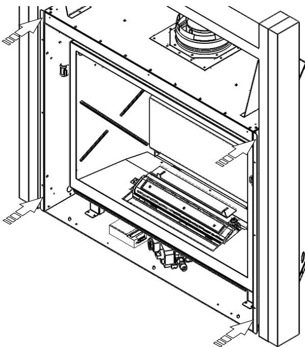
2. Install the lower panel using the three bolts at the base of the appliance (3 nuts).
