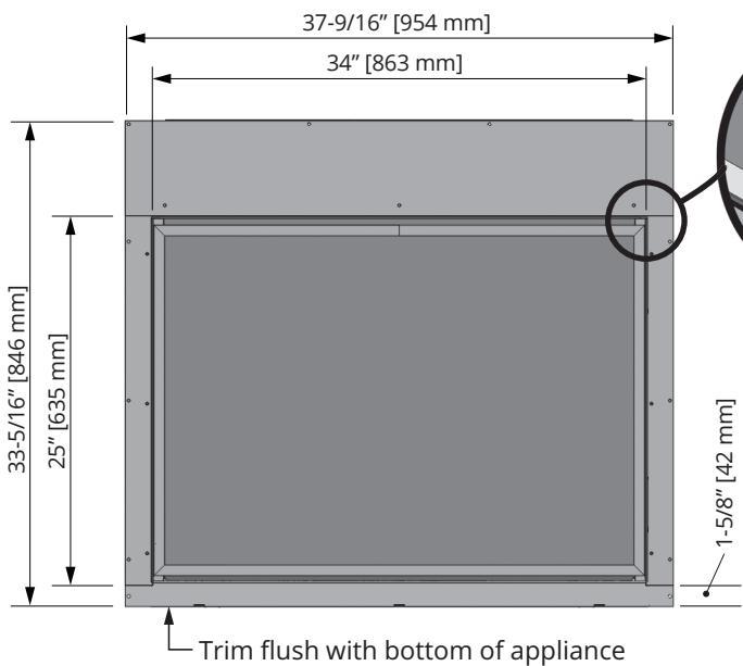
The 1030 Clean Installation Kit installs at the time of framing the appliance. Wall finishes are then applied over top of flanges and butted up to 1030's frame.
