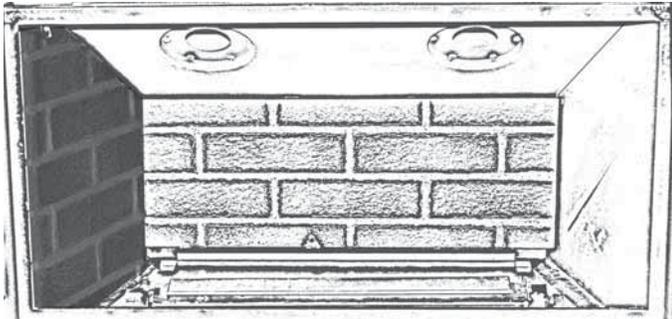
4. Rotate the anchor up and out of the way and slide the right hand side panel against the firebox side. Rotate the anchor back down to hold the panel.
