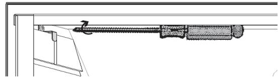
6. Install the port cover fixing it using the two screws already in the firebox top.
