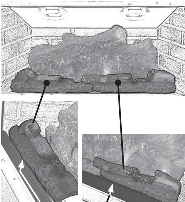
Both front logs to rest slightly on the edge of the firebox window frame.
