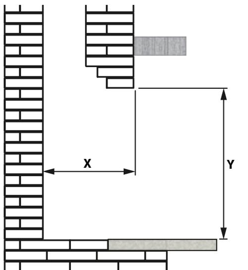
Check that masonry step does not interfere with install dimensions or vent pipe.
