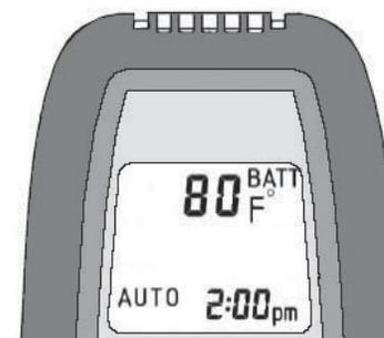
When your remote control displays **BATT**, you need to replace the battery with a new 9 volt **alkaline** battery—6LR61/MN1604.
