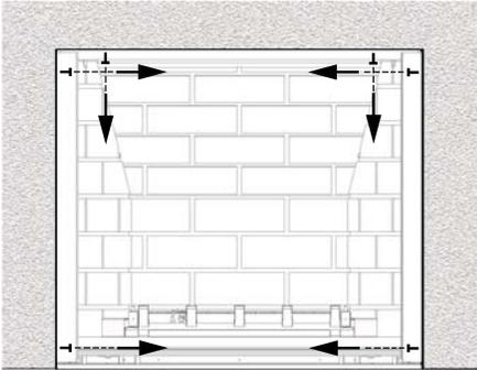
3. Install the backing plate and fix it at the top with 2 screws. Refit the overlay and fix it together with the backing plate with 1 screw on each side, as shown.
