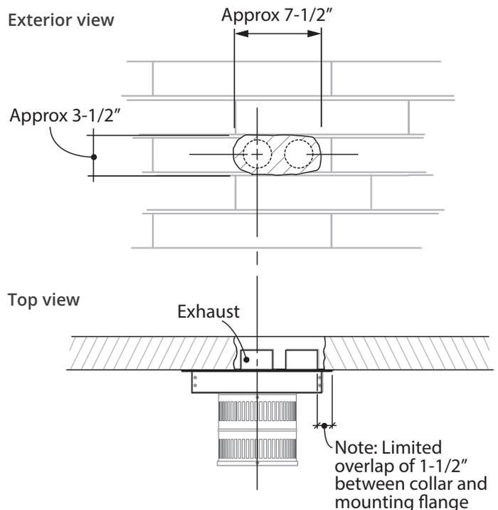
2. Rough-in approved 3-inch aluminum flex liners through the existing fireplace damper and leave enough protruding through the hole in the exterior masonry to connect terminal.
