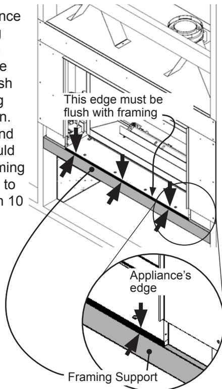
4. Fix the kit's bottom panel to the framing on each side and under the appliance's opening with 7 wood screws.
