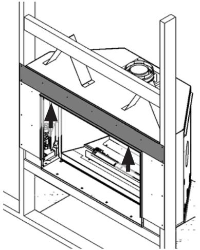
3. Slide the appliance into the framing until the bottom front edge of the appliance is flush with the framing support it sits on. The kit's side and top panels should overlap the framing studs. Fix them to the framing with 10 wood screws.
