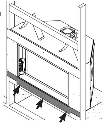
5. Fix the top, sides, and bottom pieces of cement board to the front of the appliance case with 14 screws provided.
