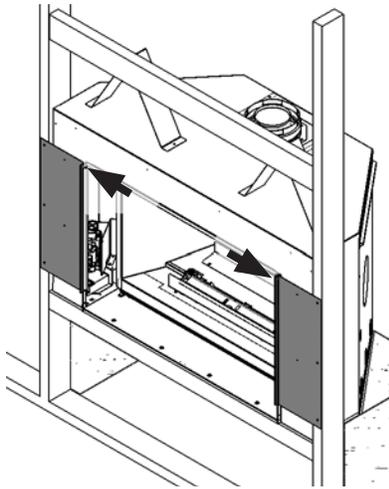
2. Slide the top panel over the flange of the top of the appliance opening. Fix the panel to the top flange with two screws.
