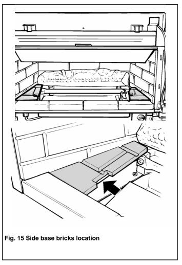
**5.4.6** Install the front log. *Be careful not to break the pegs projecting from the log.* The front edge of the log should rest behind the vertical metal edge of the firebox base which is behind the front base bricks and front burner tube. Be aware that there should be a gap between the right side of the front log and the right side base brick.
