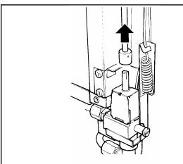
Fig. 32 Thermostat shaft disconnection
