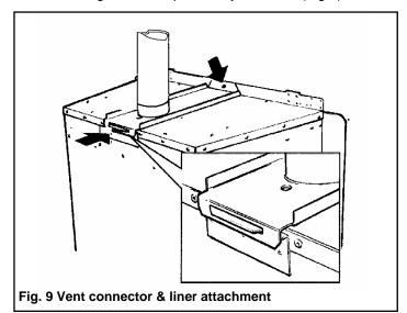
**5.2.4** Replace the top front channel and fix with the two screws previously removed. Push the appliance fully home against the front face of the fireplace. Make sure that no sags or dips occur in the liner.
