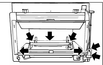
Fig. 33 Burner module disconnection points
