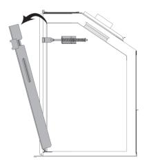
3. Lift the window out of its bottom railing and set it aside in a safe place to avoid damage.
