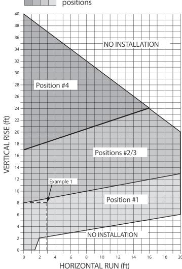
Example 1 V Value = V1 (2') + V2 (4') + V3 (2')= 8' H Value = H1 (0') + H2 (3') = 3' Restrictor position # 1 required
