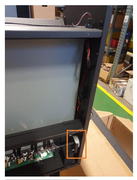
Rear spindle motor is on the left hand side of the fire and linked to the main board using 2 extension cables one goes from the motor to the top shelf and then from the top shelf to the main pcb board. The spindle motor is attached to a bracket which is fixed down by 3 screws. This spindle is plastic so don't bend and cant be bent back in to shape.
