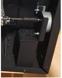
To disconnect the spindle motor you remove the spindle by pulling the spindle out of the rubber end of the motor and then unscrew the 3 screws in the base of the I shaped bracket then undo the cable connection
