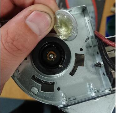
On the end of the fan unit the end that don't have a motor will have a cap on it pop it off with a flat head screwdriver and then this will expose the grease and bush make sure the bush is seated properly to allow the fan to turn freely you may want to wipe the grease off and new
