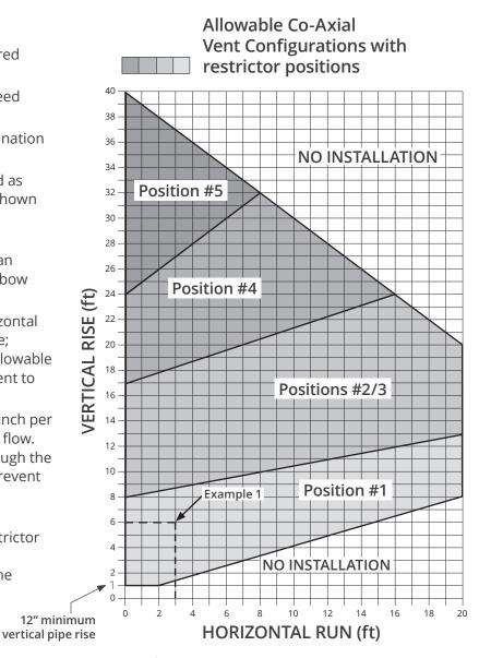
Example 1 V Value = V1 (3') + V2 (2') + V3 (1')= 6' H Value = H1 (0') + H2 (3') = 3' Restrictor position # 1 required
