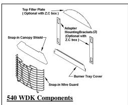
Model 540 WDK is required for all 922 Adorn Fireplace installations fitted with 539/549/550 Arch Cast fronts.
