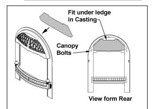
Step 3 – Install canopy shield Insert one corner of the shield into the corner behind the cast frame as shown. Bend the canopy shield to a slight radius while inserting the other corner behind the cast frame as shown (it may be necessary to loosen canopy bolts). With both the corners behind the cast frame, snap the shield forward to follow the curve of the cast iron canopy. The top of the shield should fit under the projecting ledge in the casting as shown.
