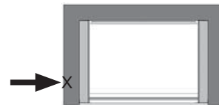
The receiver and gas valve are located on the left of the firebox behind the side door.
