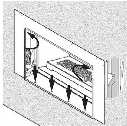
Unfasten the heater from the framing through the inside of the appliance's case on each side and at the bottom front edge.
