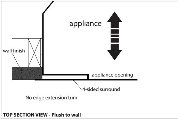
Where you want the surround flush against the finished wall, do not install the extension trim pieces. Unfasten the appliance from the framing, fit the surround to the appliance and push the appliance back into the framing cavity until the surround meets the wall. Re-fasten the appliance to the framing.
