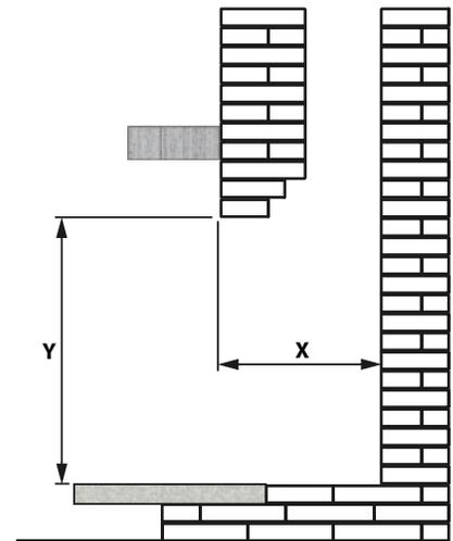
Note: Raise the G3.5 appliance by 2<sup>5</sup>/<sub>8</sub>" when using the 719BPB 4-Sided Backing Plate as the plate extends below the bottom of appliance.
